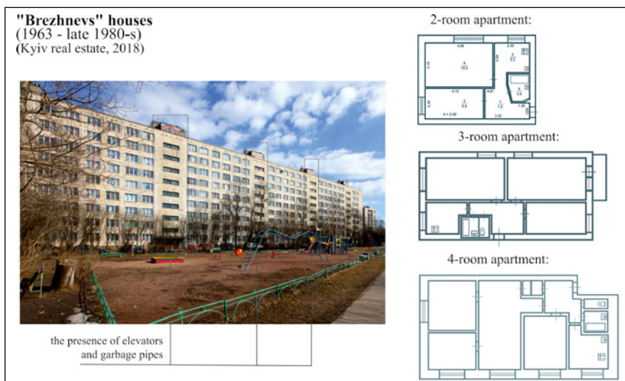
06 Characteristics of residential buildings on the Brezhnev type. © L. Shevchenko, 2018.
