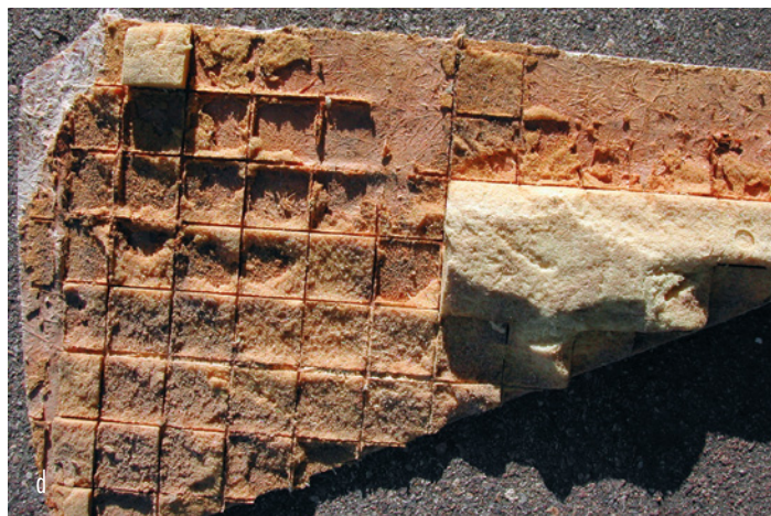
04 a - d The Futuro at the San Diego Boat Yard, damages before restoration (a) removal of green latex paint, (b) cracks and poor condition of the yellow gel coat, (c) delamination and material loss on the exterior surface, (d) removed portion from the roof area showing the rigid foam and GRP laminate. © M.W. Donaldson, October-December 2002
