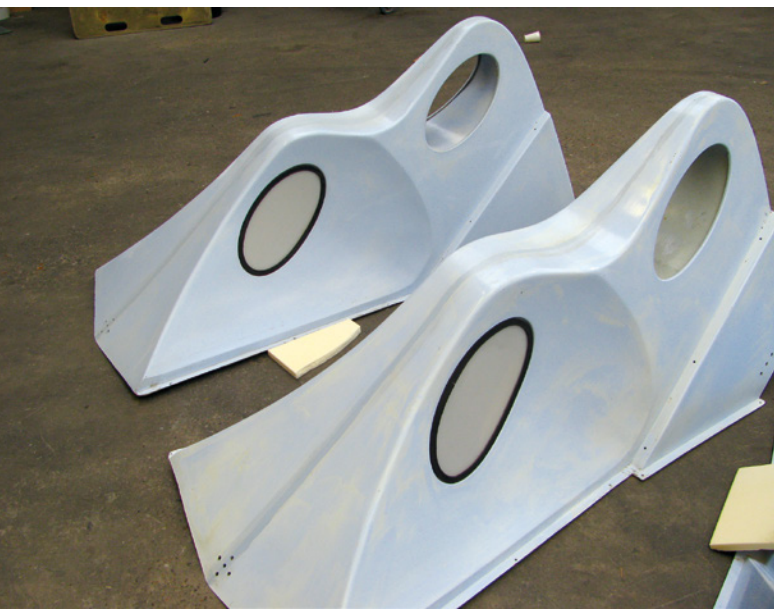
08 Two fiberglass reinforced polyester elements from the seats in the living room. © L. Beerkens
