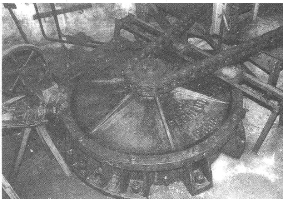
Fig. 3. Jamnagar Solarium, main axle and motor and chain in the basement/machine room bearing the "PECHUR PARIS" inscription
